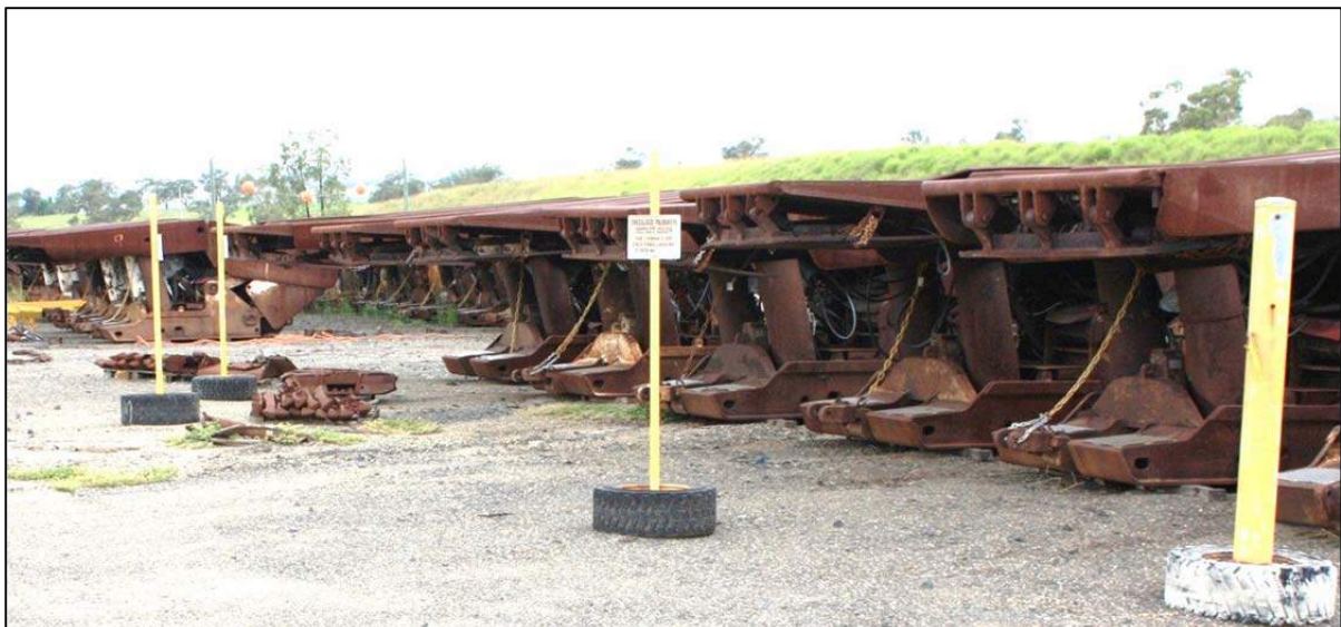
Photo 16 Longwall roof supports on the west hardstand
