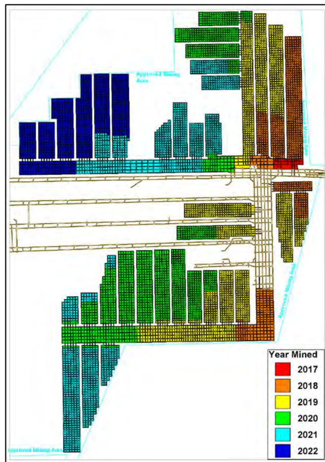
Figure 6 – Kayuga Seam Bord and Pillar Mining Sequence
