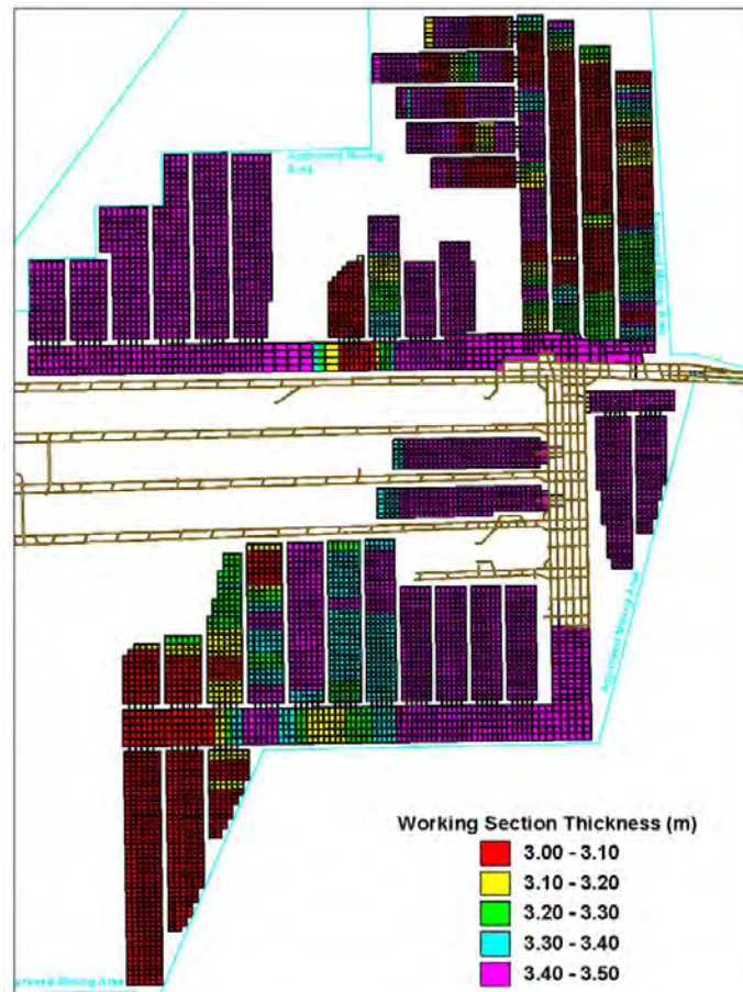
Figure 4 – Kayuga seam bord and pillar mine plan
